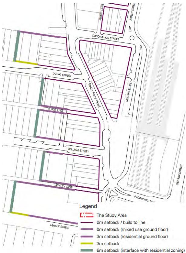
PICTURE 17 – EXISTING GROUND FLOOR SETBACKS
